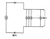
A generator G having a terminal voltage of 100 V is delivering a total current of 60 A to a load comprising N number of 50 W, 100 V lamps connected in parallel as shown in the circuit given above. What is the value of N.?
